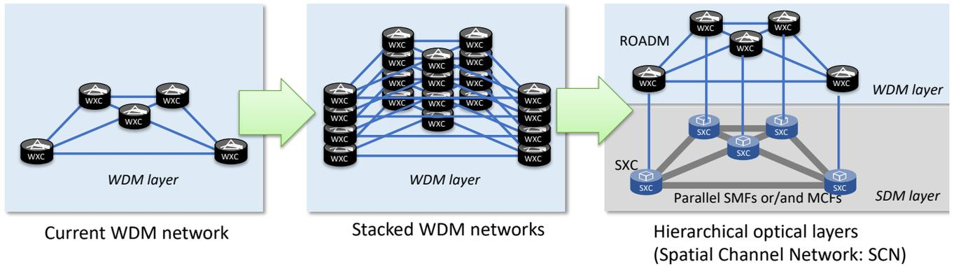
Figure 2. Evolution from WDM network to spatial channel network.
